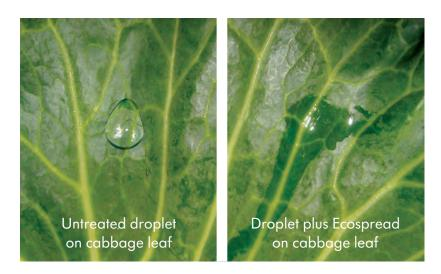
Super spreading is a consequence of lowering surface tension dramatically i.e. below 25 mN/m. Hence agricultural sprays containing ECOSPREAD® can deliver crop protection products and foliar fertiliser more effectively by:
